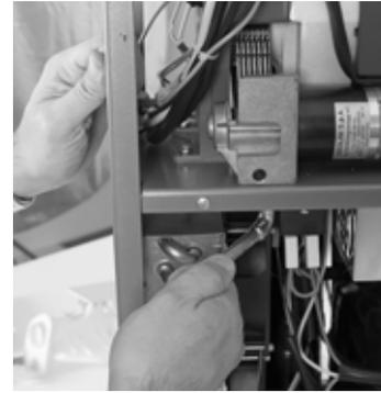
2 Unscrew the 6 pulley support screws, positioned as follows : 2 lower, 2 central and 2 upper.
