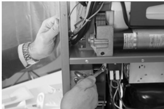
2 Set the tension of the belt using the screw located on the gear motor support. Turning it clockwise the tension of the belt is
