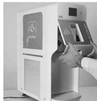
3 Insert the USB key into the appropriate port located as shown in picture. Start the dispenser by simultaneously actuating the
